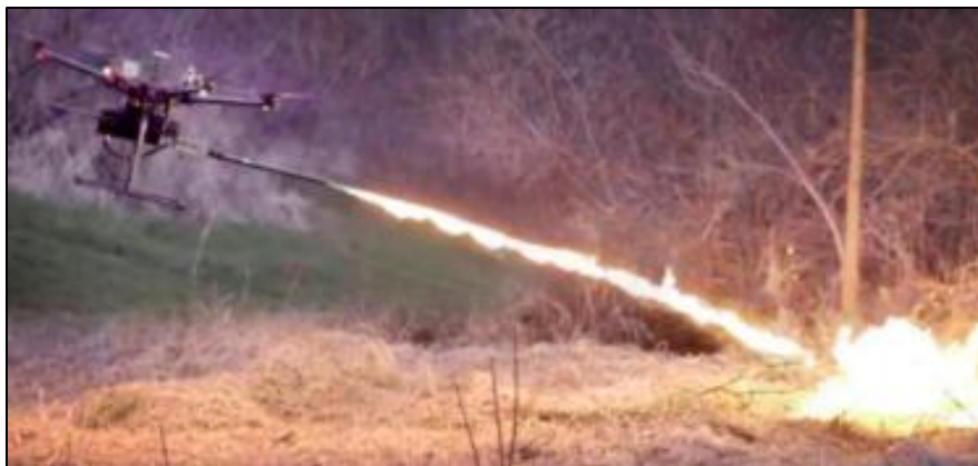
Commercially available “flame thrower” UAS marketed for landscaping and wasp removal
