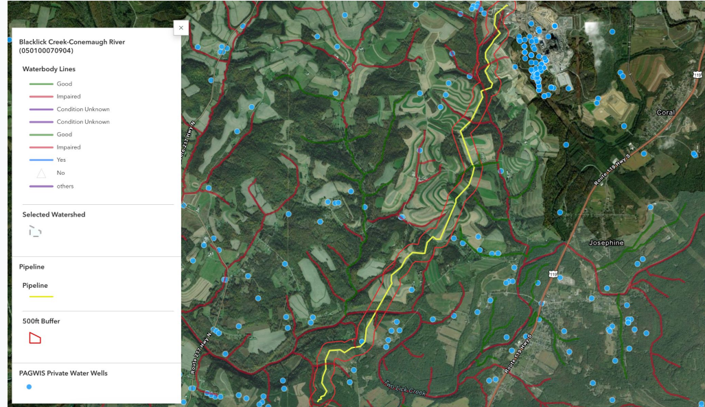
Pipeline route, watershed boundary, and nearby private water wells within the 500-ft construction buffer. Source: PA Groundwater Information System, EPA My Waterway.
